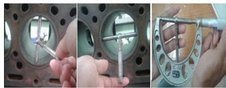
Gambar 7. Pengukuran liner Cylinder
