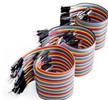
Gambar 8. Kabel Jumper Sumber: Dokumentasi penelitian, 2024
