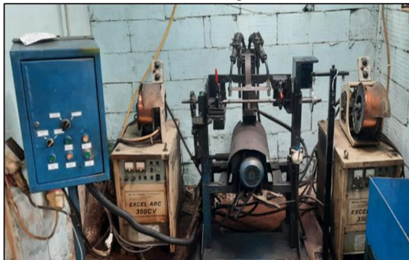
Gambar 17. Automation Machine Welding
